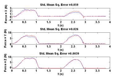
**Figure 3:** Predicted (red) force vectors (Z = normal, X, Y = tangential) compared to actual forces (blue) for two of a set of manual contacts with the BioTAC. More systematic datasets for regression and validation are now being generated by contact with various probes controlled by a stepper-motor.
