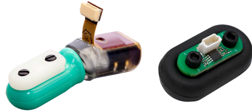
Figure 1: Left - a BioTac® tactile sensor; Right - a low-cost NumaTac® prototype tactile sensor.
