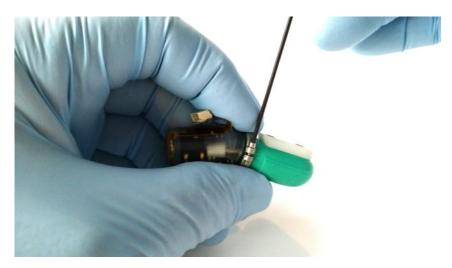
**5.** Tighten each screw until the split rings are flush with each other, readjusting if there is nail silicon pinched in between the plastic and the ring.
