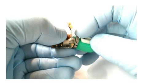
**4.** Insert 1 screw (0-80) through one of the holes of the top split ring and screw only a couple of threads into the bottom split ring. Alternate between either side, progressively tightening equally
