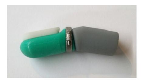
In this photo the split ring is correctly aligned along the top piece of the ring but the bottom ring piece is incorrectly placed too far away from the body of the BioTac. The screws have been correctly tightened to allow the two ring pieces to touch.
