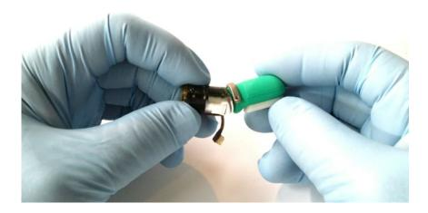
**3.** Place the non threaded half of the split ring on the top of the BioTac skin taking care to align the holes
