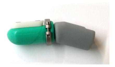
In this photo, the split ring is incorrectly aligned with the nail and is not flush with the plastic of the body of the BioTac. The screws also need to be tightened so that the two pieces meet.
